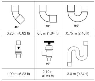
Tab. 4: Equivalent length for external diameter 12 mm (0.5")
