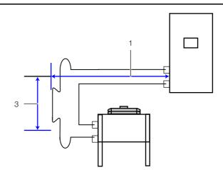
Fig. 14: Relative positioning – condenser below the LCP DX
