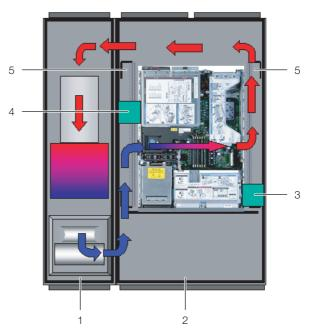
Fig. 17: Placement of foam strips for devices with sideways air throughput (top view) – LCP Rack DX
