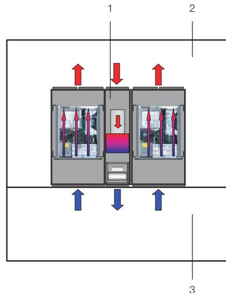
Fig. 15: Installation room with cold aisle containment
