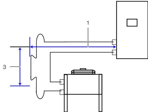
Fig. 14: Relative positioning – condenser below the LCP DX
