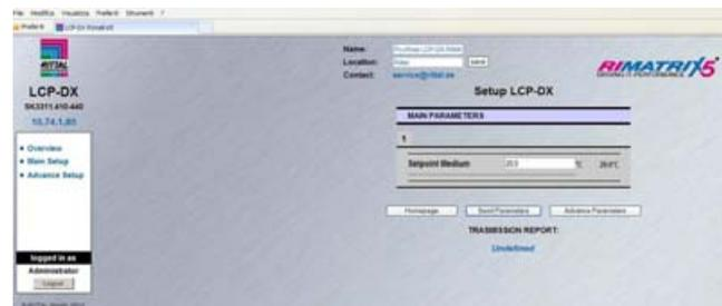
Fig. 38: Setting the server air injection temperature
