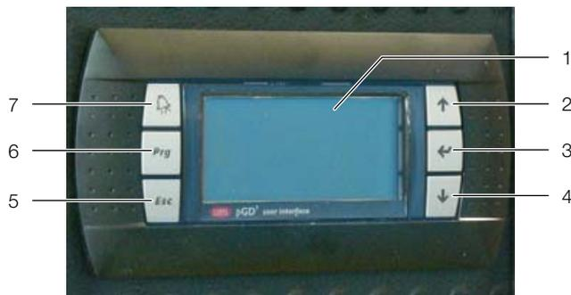
Fig. 39: Control and display components
