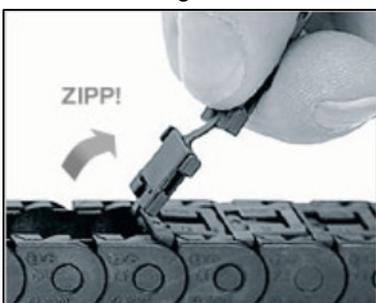
Remove the screws at the rear connection panel (3), disconnect the VGA-cable on device side. Remove the cable from the energy chain. Mount the supplied DVI cable in the opposite sequence. Close the cover of the energy chain.
