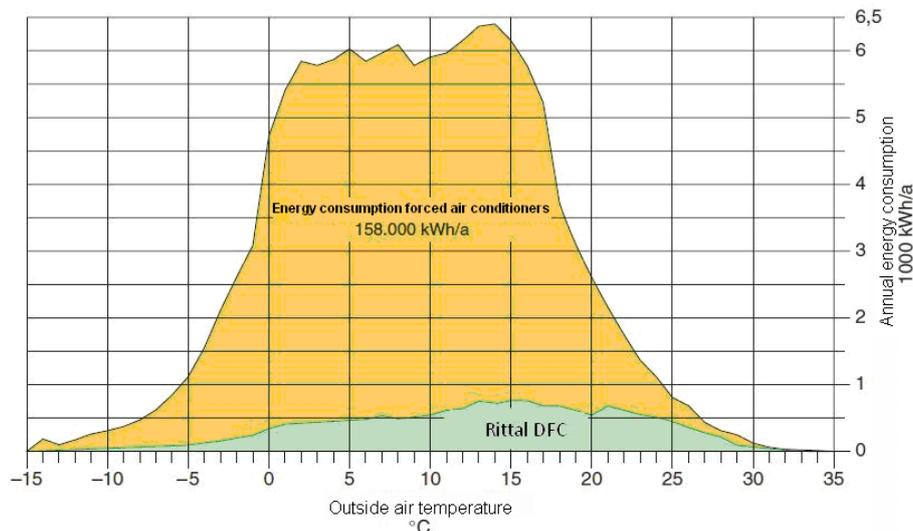
**Figure 6: Annual energy consumption of circulating systems and direct free cooling**
