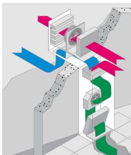
**Figure 5: Direct free cooling**
