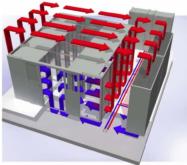
**Figure 2: Function principle of cold aisle containment**
