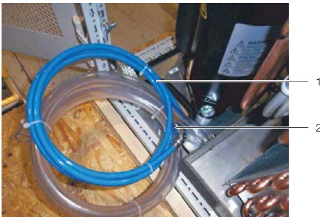
Fig. 50: Connection hose with \frac{1}{8} " external thread adapter
