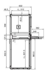
1 Max. 504.5, adjustable on a 25 mm pitch pattern i.L. = Clearance width
