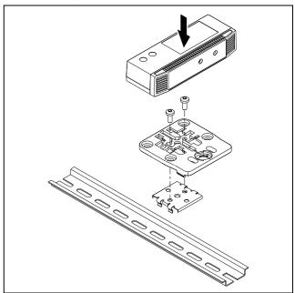
Fig. 8: Fastening the bracket to the spring clip
