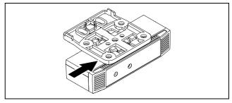
Fig. 4: Latching the sensor into place on the bracket
