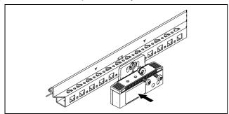
Fig. 6: Optional securing of the bracket
