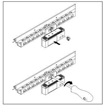
Fig. 5: Mounting the sensor in the enclosure or IT enclosure
