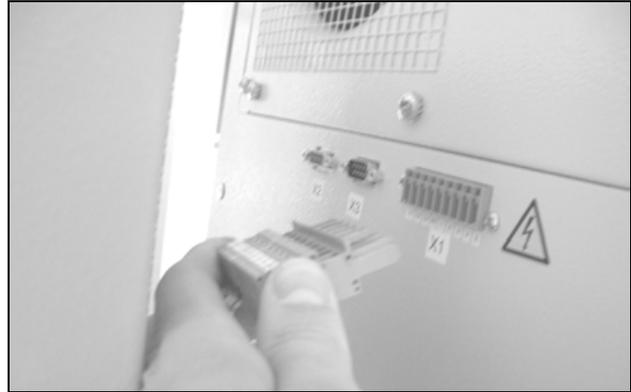
Fig. 53: Disconnect the mains plug
