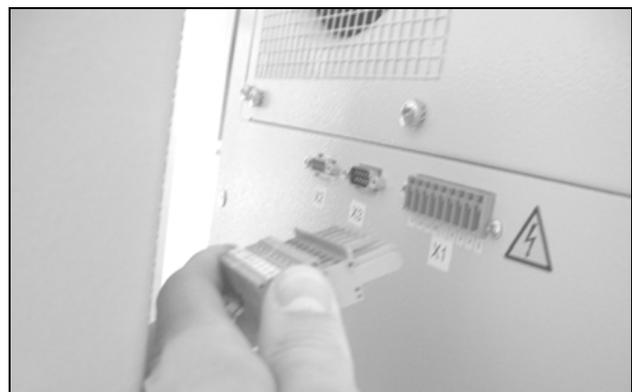
Fig. 34: Disconnect the mains plug
