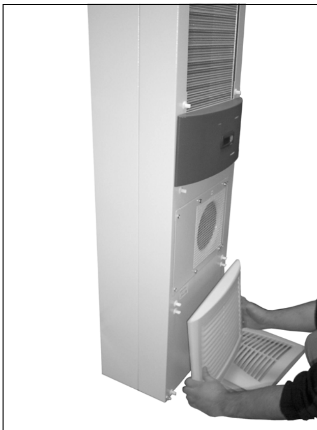
Fig. 58: Remover a grade inferior (2)
