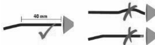
Fig. 14: Insert the wire correctly
