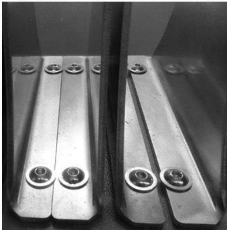
Fig. 5: Reel holder (length 8 mm: left, length 10 mm: right)
