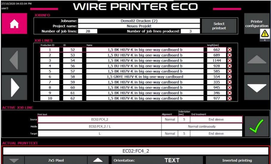
The screenshot displays the control interface for the WIRE PRINTER ECO. At the top, it shows the date and time (27/10/2020 04:03:04 PM) and the user (user3). The main section is titled "JOBINFO" and contains fields for Jobname (Demo02 Drucken (2)), Project name (Neues Projekt), Number of job lines (28), and Number of job lines produced (3). There is a "Select printset" button and a "Printer configuration" icon with a warning symbol.
