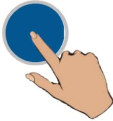
Once the Emergency Stop push-button has been unlocked, safety must be acknowledged by pressing the blue Reset push-button.
