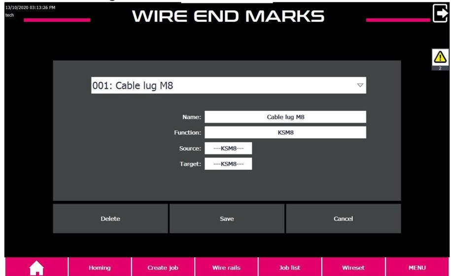
Machining marks are overprints at the wire start or wire end that can be selected instead of an end treatment. The overprint is maximum 10 characters and provides information about the end treatment to be applied.
