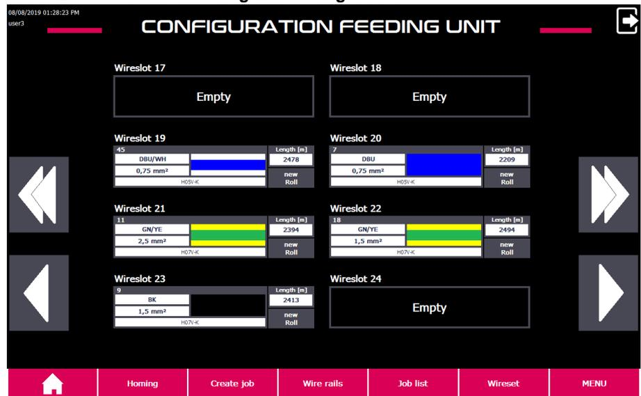
This menu sets up wires, specifies new rollers for setup wires and removes wires from the wire slot. Depending on the variant, 24 or 36 wires can be setup concurrently.
