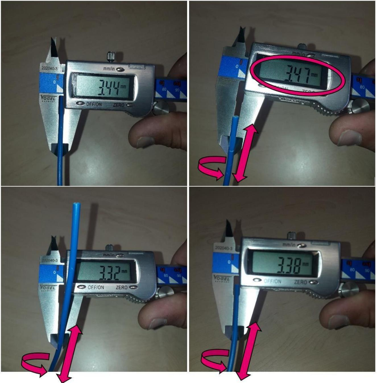
Check the wire diameter at at least three positions of the wire. Because wires do not have an absolutely cylindrical form, the wire must also be turned radially at the various measurement positions. The largest measured value is taken as the wire diameter.
