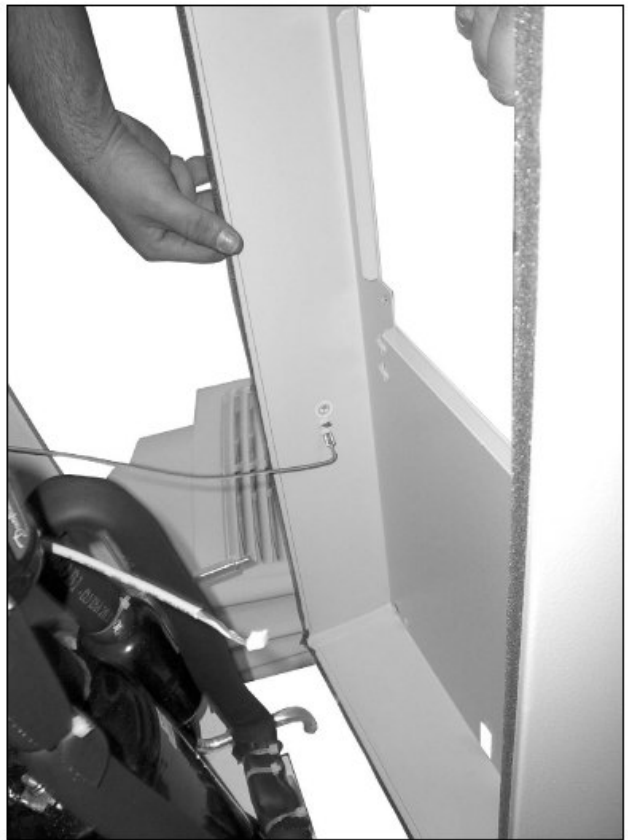
图77: 断开接地电缆 (1)
