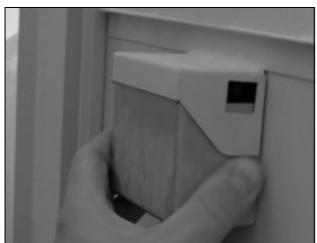
Fig. 14: Release the cover plate
