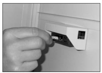
Fig. 29: Disconnect the connector from the display
