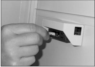
Fig. 15: Connect the display connection cable
