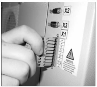
Fig. 28: Disconnect the mains plug
