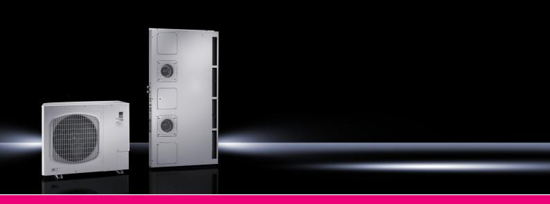
The cooling unit with inverter technology allows targeted speed control of the compressor. The coolant volume is regulated via the electronic expansion valve. Adaptation to cooling requirements facilitates energy savings of up to 40%. The cold air is expelled in front of the 482.6 mm (19") level by the internal unit (evaporator coil), while the hot air is drawn in at the rear.
