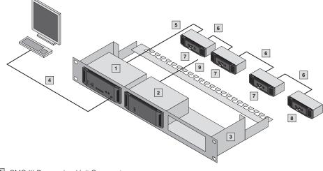
1 CMC III Processing Unit Compact (with front infrared access sensor, temperature sensor, 2/1 inputs/outputs)
