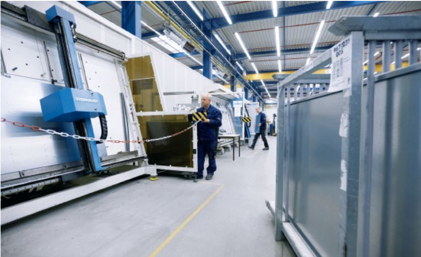
ATR has Rittal supply its enclosures in separate parts. In addition to saving on dismantling time and packaging material, this also makes production more flexible.
