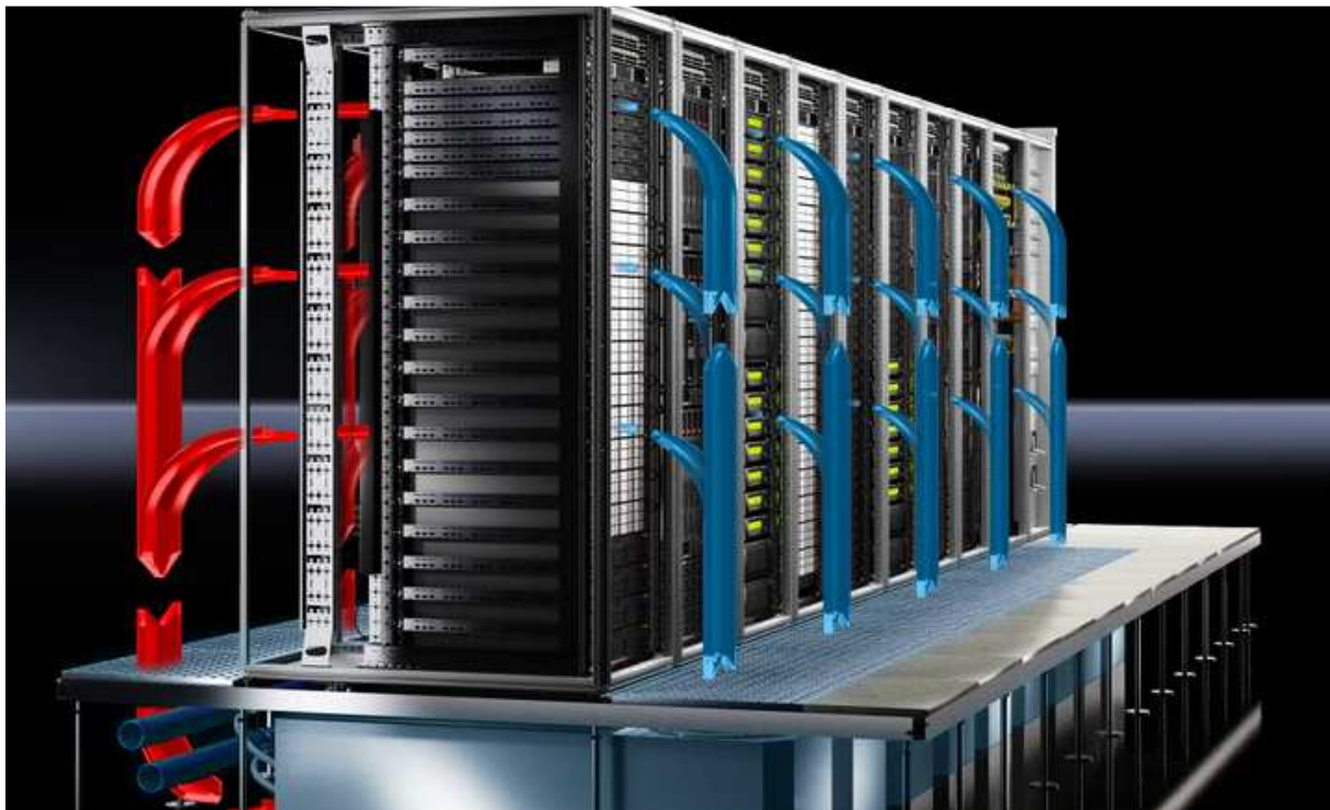
Figure 5: Air routing of the server modules
