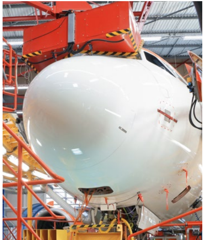
DIGITAL VIEW No stunning aerial vista for the engineers: Monitors are mounted in front of the cockpit to display the ground test instructions.
