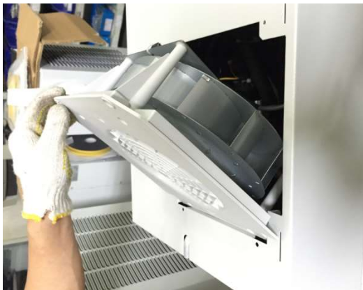
Figure 21: Remove the outside fan
