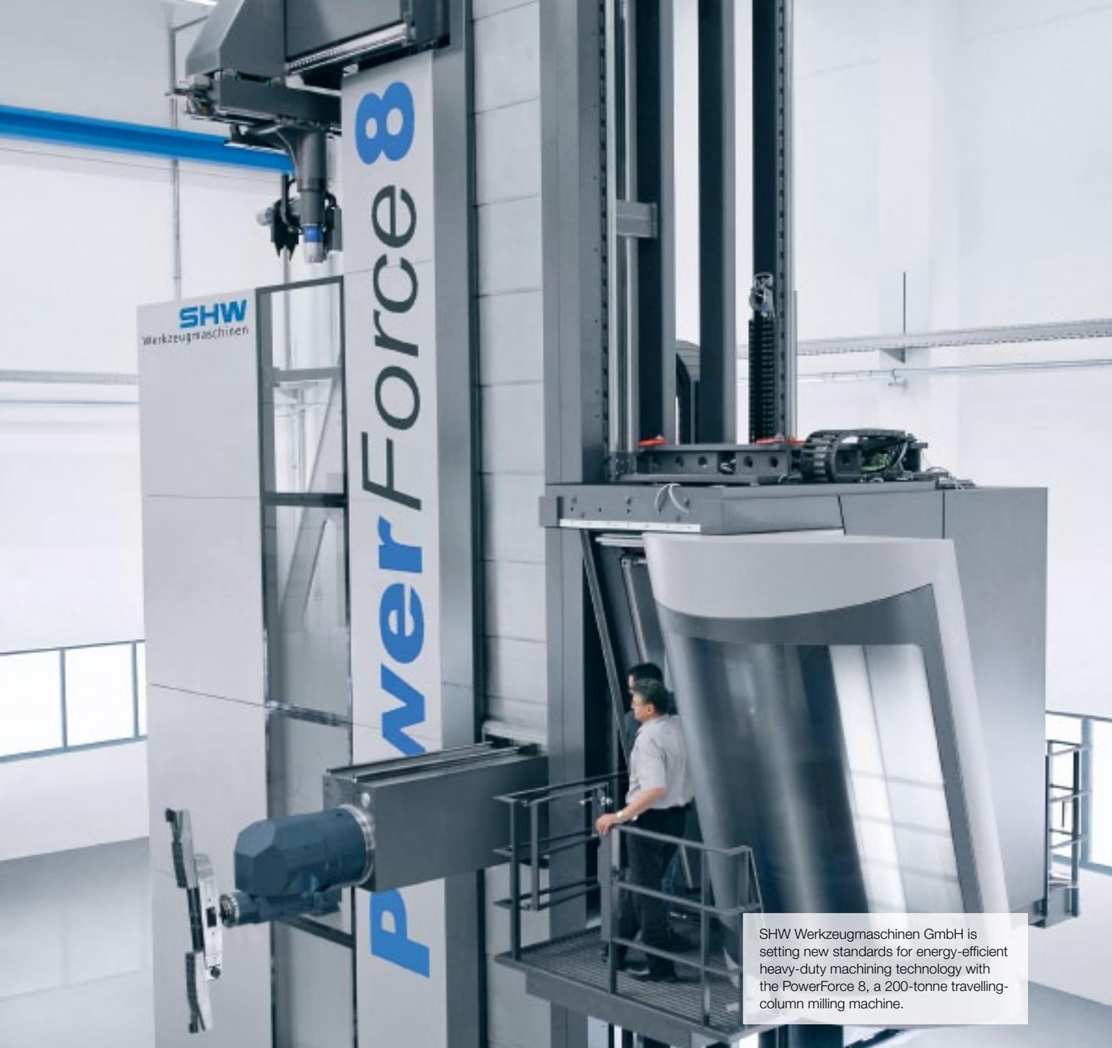
SHW Werkzeugmaschinen GmbH is setting new standards for energy-efficient heavy-duty machining technology with the PowerForce 8, a 200-tonne travelling-column milling machine.
