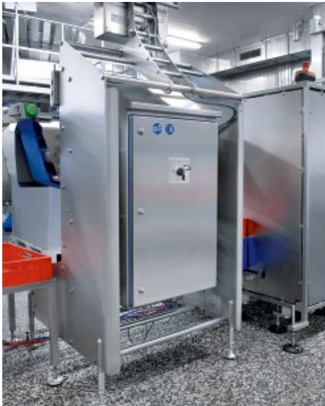
Special Hygienic Design technology from Rittal makes Bizerba's new dynamic check-weigher ideal for use in the food industry. It checks the weight of the goods to be packaged at high speed.
