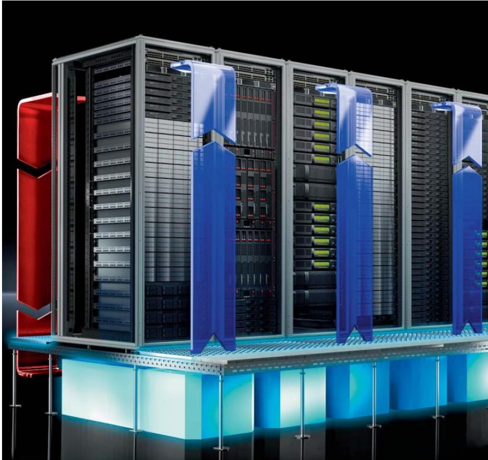
Figure 7: Climate control for the server module
