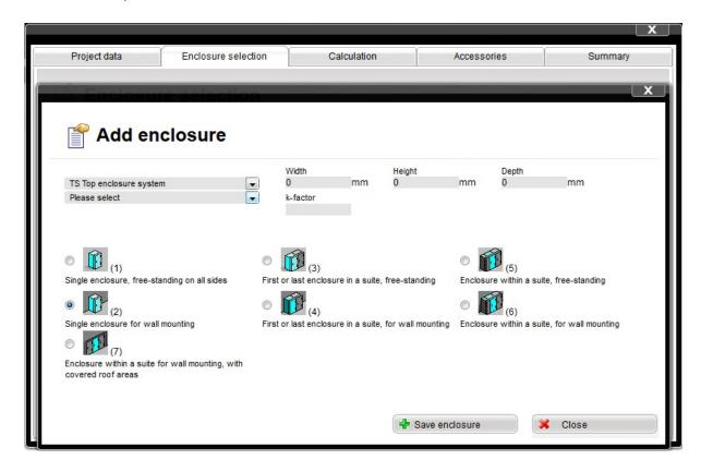
When you click the "Save housing" button, a message box prompts whether the heat loss data is to be assigned to the selected housing. If no data is to be entered, you must select "Cancel". When you click "OK", a new window opens with three tabs:
