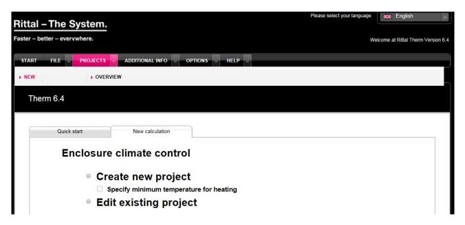
You can configure an enclosure heating in the "Specify minimum temperature for heating" menu item.
