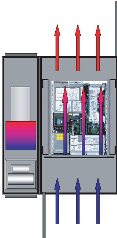
If the need arises, both the front and the rear door are automatically opened. The air flows unhindered into the interior of the enclosure, circulates around the installed equipment and exits the system via the open rear door of the enclosure. It is important to ensure that the LCP fans are switched off, otherwise hot air will be blasted in front of the 482.6 mm (19") level in the event of emergency cooling.
