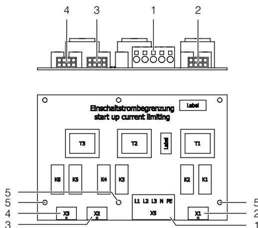
Fig. 93: Startup current limitation – rear/top view
