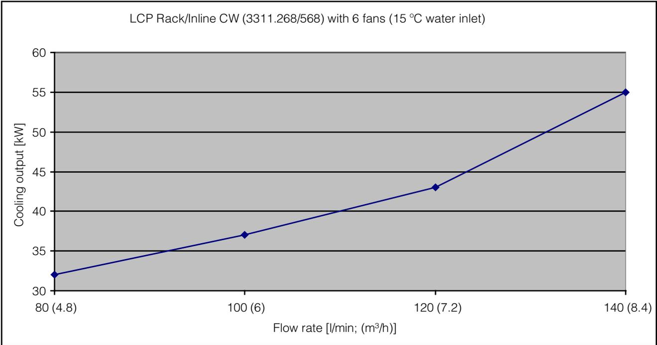
Fig. 84: Cooling output of the LCP Rack/Inline in the "60 kW" version with six fans
