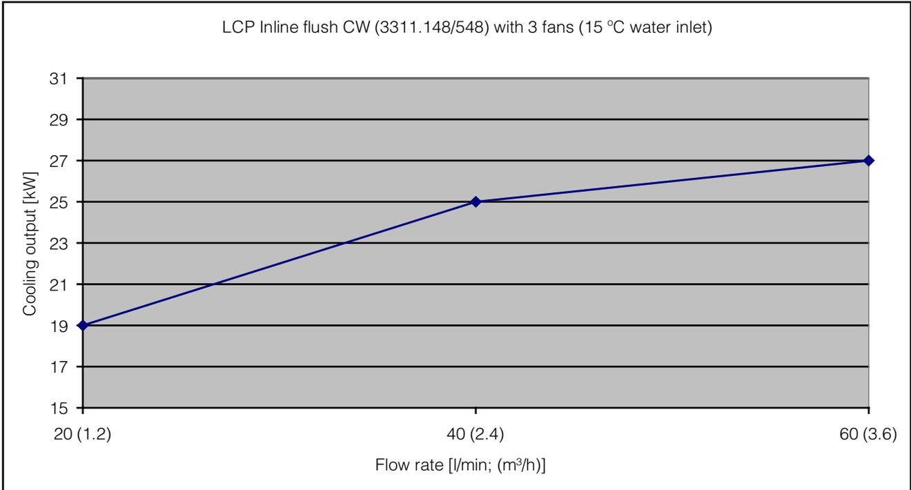
Fig. 80: Cooling output of the LCP Inline flush with three fans
