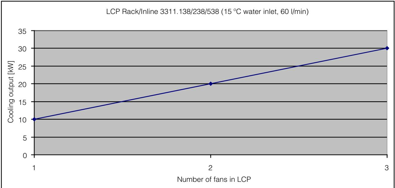
Fig. 78: Cooling output of the LCP Rack/Inline in the "30 kW" version
