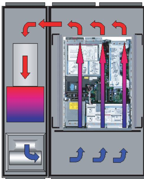
Fig. 95: "Front to back" cooling principle with bayed LCP Rack
