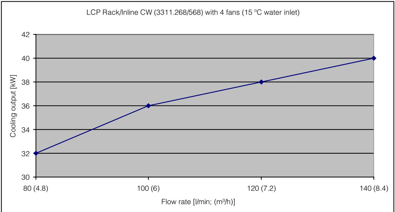
Fig. 82: Cooling output of the LCP Rack/Inline in the "60 kW" version with four fans
