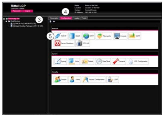
Fig. 49: Adjusting the TCP/IP settings
