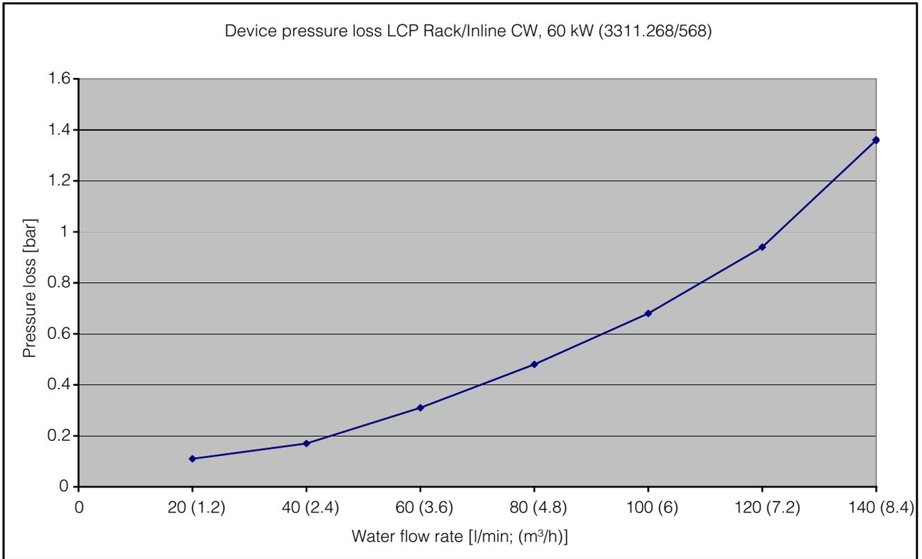
Fig. 86: Pressure loss of the LCP Rack/Inline in the "60 kW" version
