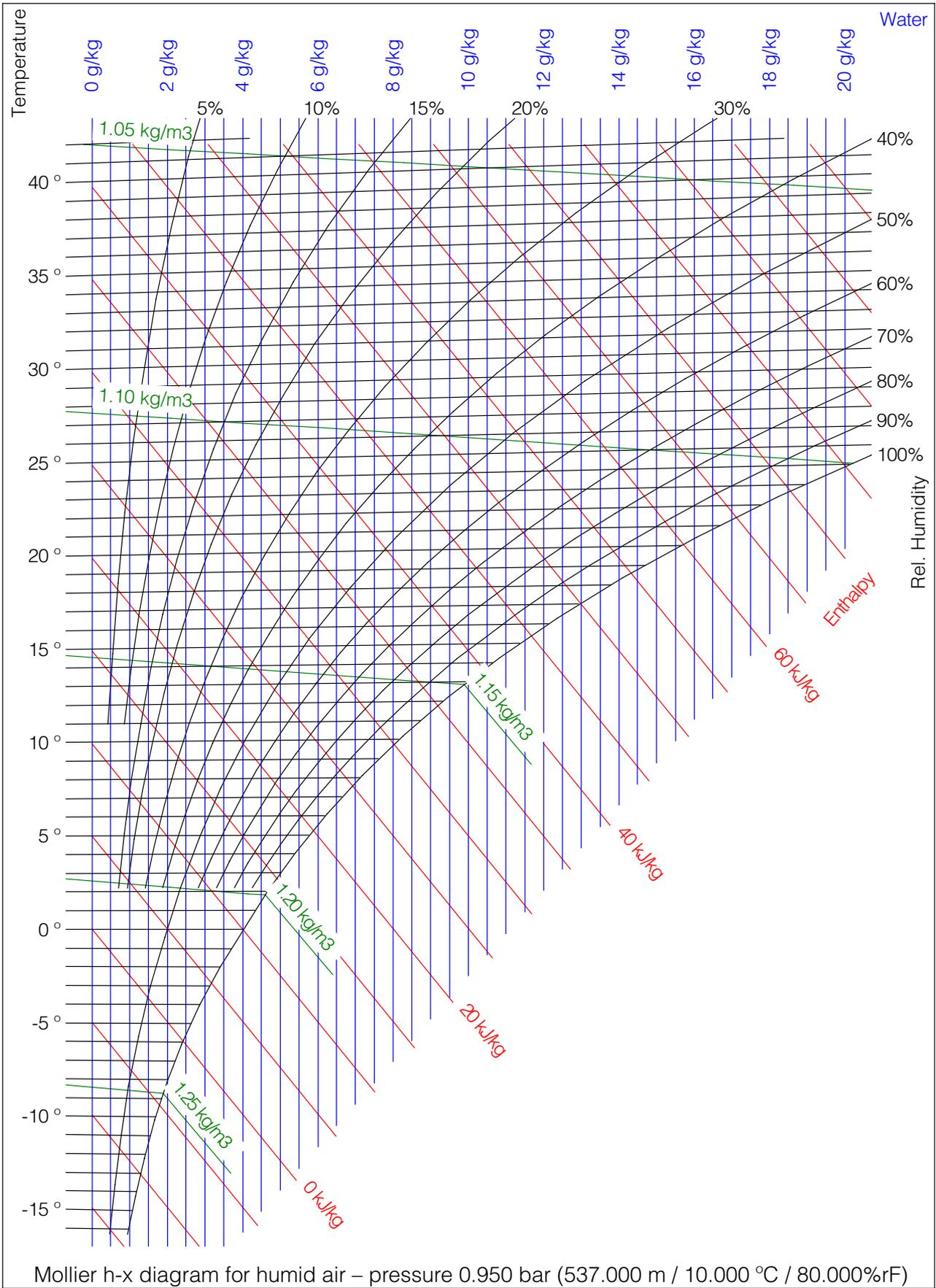
Fig. 4: Mollier h-x diagram for humid air
