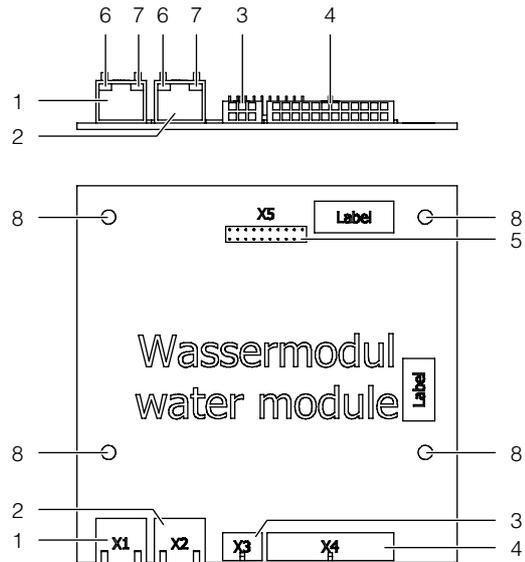
Fig. 92: Control unit water module – rear/top view
