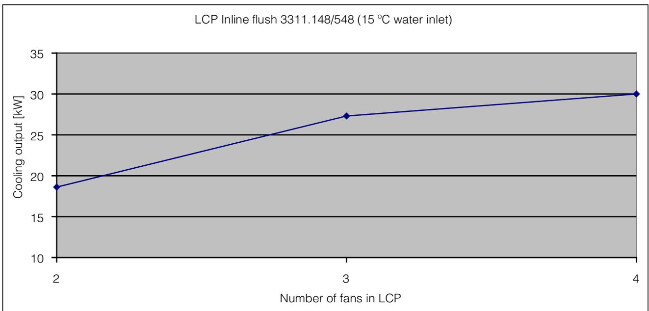
Fig. 79: Cooling output of the LCP Inline flush
