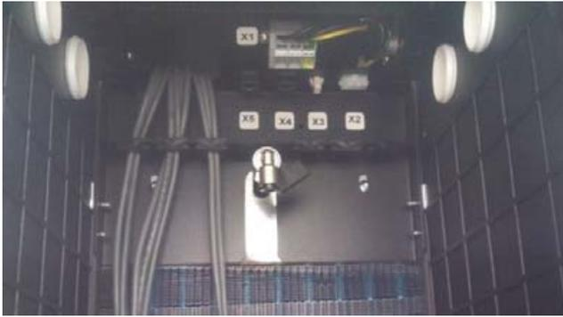
Fig. 39: Terminal connections X1–X5 without access panel
