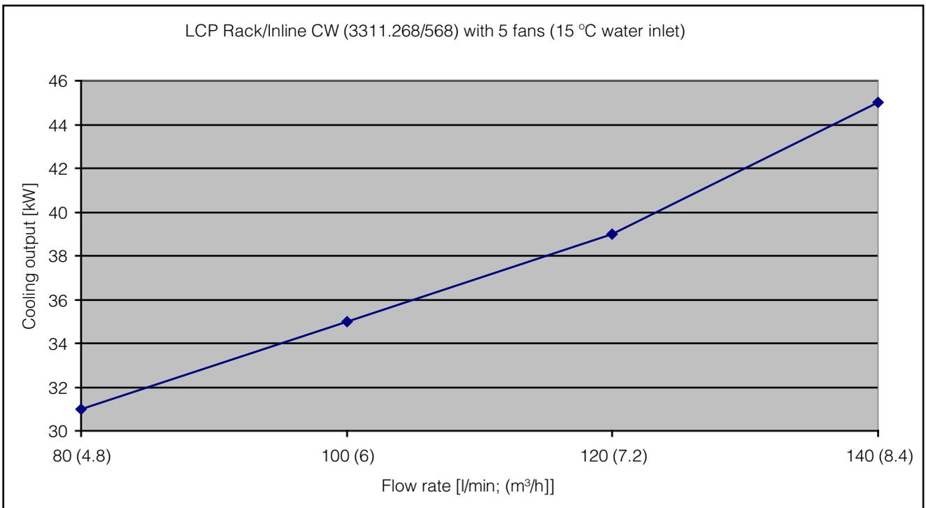
Fig. 83: Cooling output of the LCP Rack/Inline in the "60 kW" version with five fans
