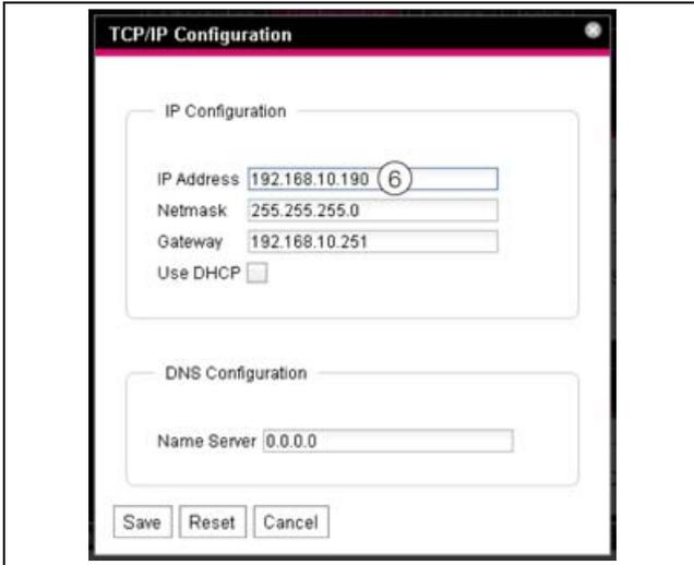
Fig. 50: Adjusting the TCP/IP settings
