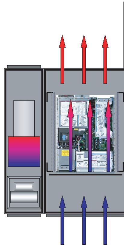
If the need arises, only the rear door of the enclosure is automatically opened. The air flows into the interior of the enclosure via the perforated front door, circulates around the installed equipment and exits the system via the open rear door of the enclosure. It is important to ensure that the LCP fans are switched off, otherwise hot air will be blasted in front of the 482.6 mm (19") level in the event of emergency cooling.
