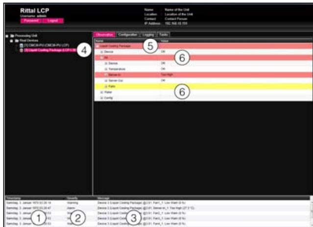
Fig. 68: Layout of message display
