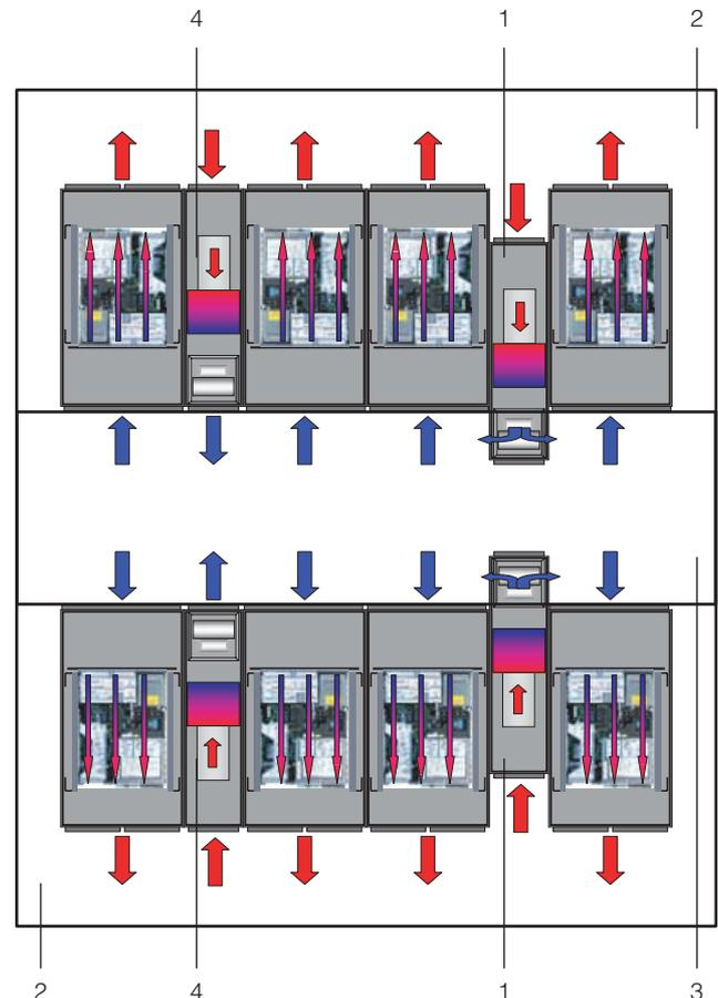
Fig. 20: Installation room with cold aisle compartmentalisation
