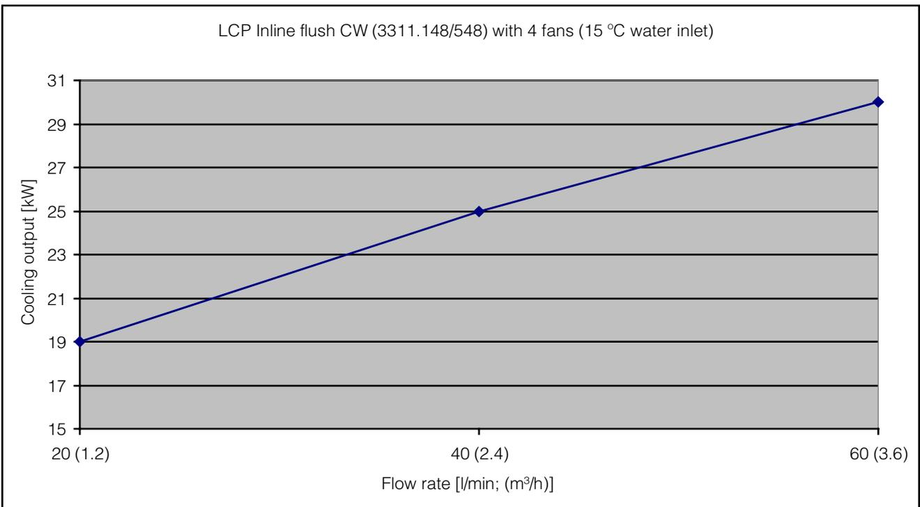
Fig. 81: Cooling output of the LCP Inline flush with four fans
