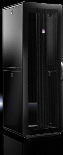
TS IT Pro configured for ready deployment. Enclosures are complete with depth adjustable 19" EIA rails, casters, right and left cable management walls each with dual PDU mounting, baying kit and locking front and rear perforated doors. Available in a range of sizes with sidewalls.
