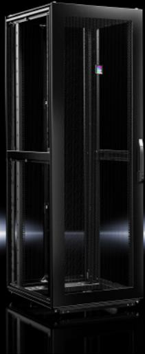
TS IT Pro configured for ready deployment. Enclosures are complete with depth adjustable 19" EIA rails, casters, cable management walls with dual PDU mounting, baying kit and locking front and rear perforated doors. Available in a range of sizes without sidewalls.
