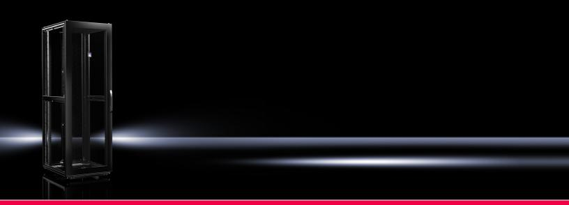
TS IT Pro configured for ready deployment. Enclosures are complete with depth adjustable 19" EIA rails, casters, cable management walls with dual PDU mounting, baying kit and locking front and rear perforated doors. Available in a range of sizes without sidewalls.
