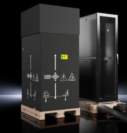
TS IT Pro configured for ready deployment. Enclosures are complete with depth adjustable 19" EIA rails, casters, right and left cable management walls each with dual PDU mounting, baying kit and locking front and rear perforated doors. Robust packaging system designed for safe equipment integration, transportation, and on site deployment. Meets ISTA 3E standards. Available in a range of sizes with sidewalls.
