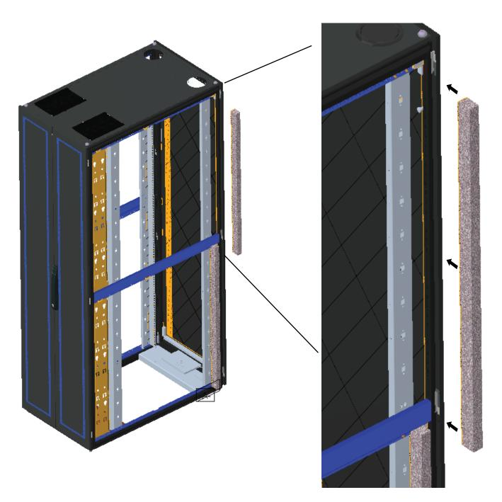
FOAM BAFFLE INSTALLATION INSTRUCTIONS BAYING BETWEEN RAIL CONFIGURATION
