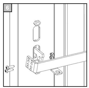
It must be ensured that the defeater lever and the screws are attached to the disconnect tab from the left.
