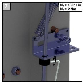
The lower collet is fixed with the supplied 1.5 mm Allen key.
