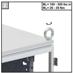
Rotate each of the 4 eyebolts so that they are parallel with the left and right sides of the enclosure.
