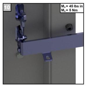
Only for configuration option 4: then the defeater lever can be attached to the adapter bracket Siemens. The mounting holes must be selected as shown in Figure 5!
