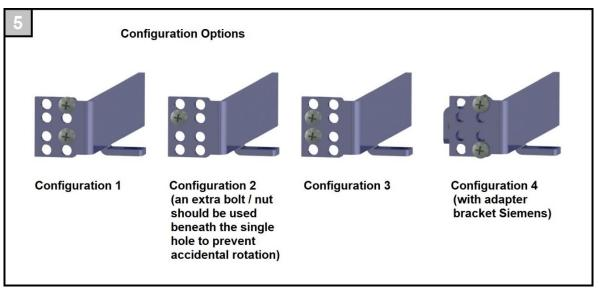
Caution! If the mounting holes shown here are not used when mounting the defeater lever on the disconnect handle, the system will not function properly!
