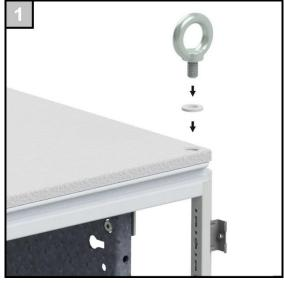
Ensure the rubber washer is set over each of the 4 eyebolts.
