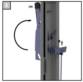
Turn the disconnect handle to the 'ON' position by pushing down on the defeater lever.
