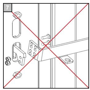
The assembly of the defeater lever and the screws from the right is not permitted!
