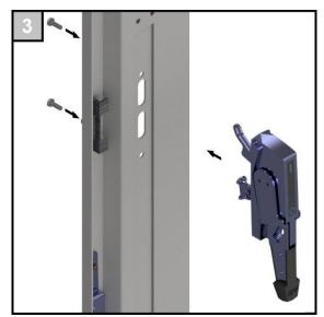
The disconnect handle (not supplied with the enclosure) is mounted according to the manufacturer's specifications. For Attachment use manufacturer's hardware.
