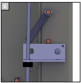
Position the lower collet just below the activator bracket.
