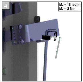
The upper collet is fixed with the supplied 1.5 mm Allen key.
