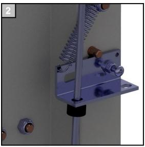
Then the connecting rod must be pushed through the activator bracket and then through the second collet.
