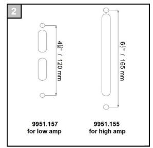
Adapter plate 9951.157 with universal cutout for low amp disconnects-standard or adapter plate 9951.155 with universal cutout for high amp disconnects-standard.
