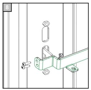
The special defeater levers for switches from Eaton and LSIS must also be installed from the left.
