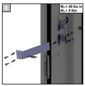
The defeater lever is attached to the disconnect handle as described on the following pages. If the handle has threaded holes, use manufacturer's hardware. If the handle has thru-holes, use Rittal M4x12 screws and M4 nuts.
