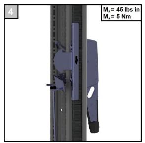
When the disconnect handle is switched to "OFF", the defeater lever is lowered so far that it is no longer blocked by the door catch. The door can be opened. Then the screws of the door catch must be tightened.
