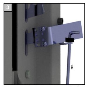
The connecting rod must be pushed down as far as possible.
