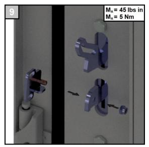
Only for configuration option 4: the adapter bracket Siemens is first mounted on the disconnect handle.
