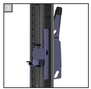
When the disconnect handle is switched 'ON', the door catch is positioned and tighten on the master door stiffener above the defeater lever so that the master door is effectively locked and opening is prevented.
