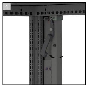
The FMDC door must be closed and fully latched at the top and bottom. The screws of the door catch need to be loosened a little.
