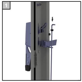
The connecting rod must be pushed from above through the first collet and the hole in the tab of the defeater lever.
