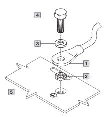
PE conductor with ring terminal
