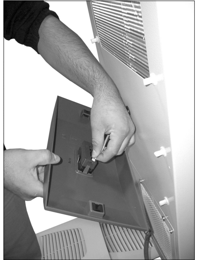
Fig. 45: Disconnect the connector from the display (1)
