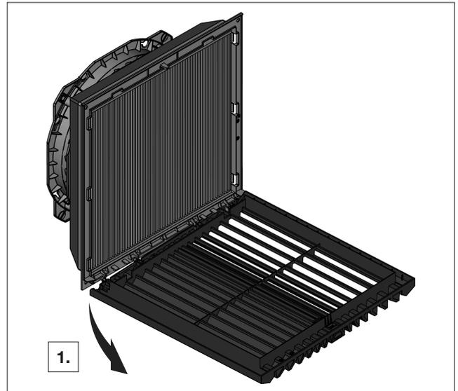
Fig. 5: Release the l/h side of the louvred grille hinge (3239.xxx to 3244.xxx)
