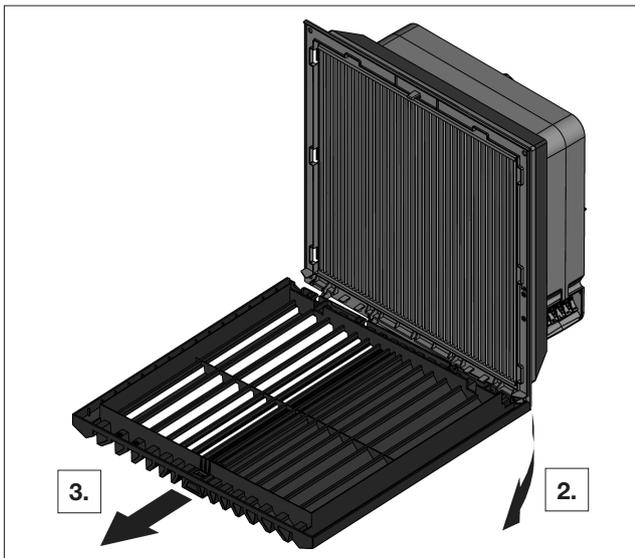
Fig. 4: Release the r/h side of the hinge and remove the louvred grille
