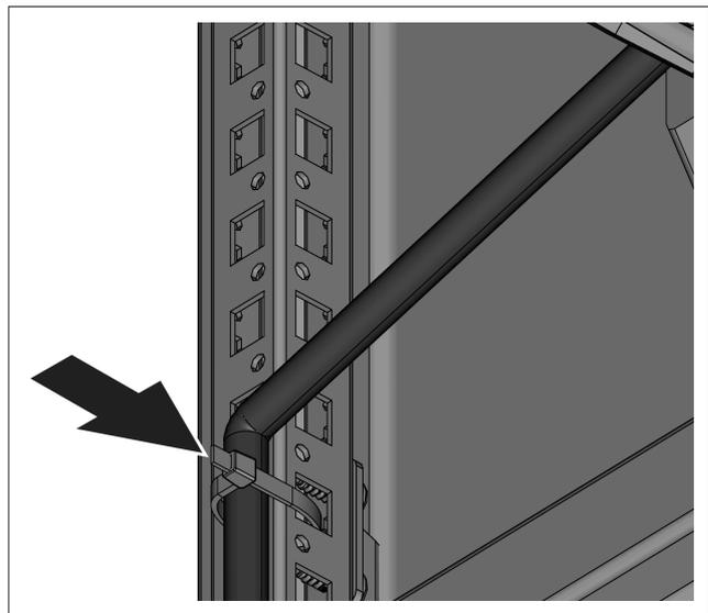
Fig. 8: Cable fastening with cable ties on the enclosure frame (example)
