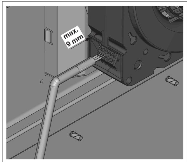
Fig. 7: Maximum permissible insulation stripping
