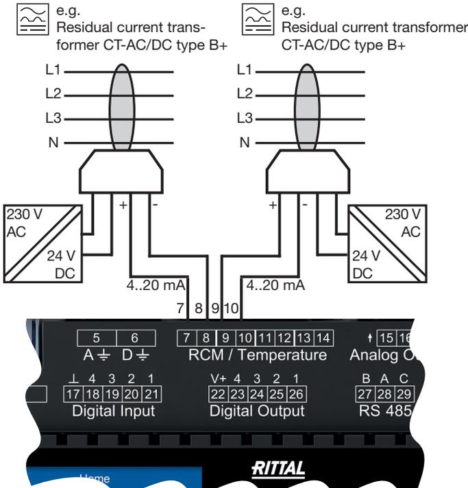
Fig. Connection variant, residual current measurement using a current transformer of Type B. Each residual current transformer of the series CT-AC/DC type B+ RCM requires its own power supply (with  $U = 24 \text{ VDC}$ , residual ripple  $< 5\%$ , power = 24 W).
