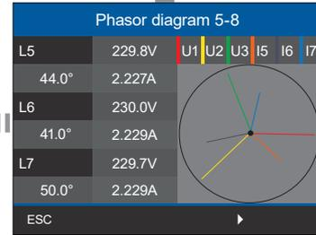
Display, Voltage L5, L6, L7; current L5, L6, L7; phase shift between voltage and current L5, L6, L7.
