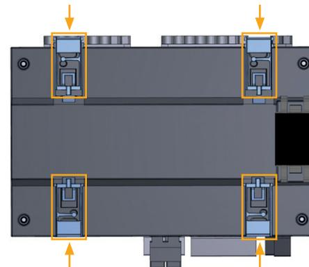
Fig. 4 - Pushing in the bottom bolts:
