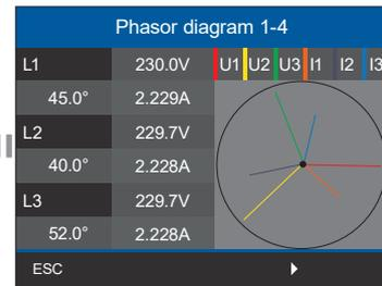
Display, Voltage L1, L2, L3; current L1, L2, L3; phase shift between voltage and current L1, L2, L3.
