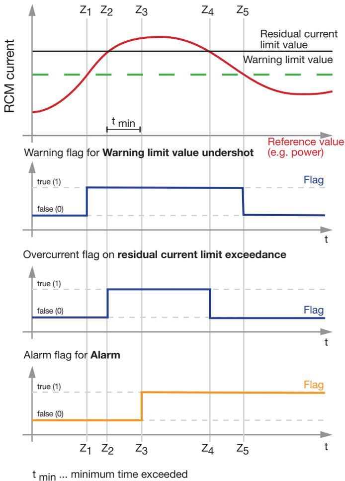
The adjacent graphs explain the 3 events **Warning limit exceeded**, **Residual current limit value exceeded** and **Alarm flag** with the states:
