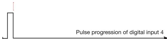
Fig.: Principle of the pulse sequence at digital input 4 - falling edge
