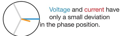
Voltage and current have only a small deviation in the phase position.
