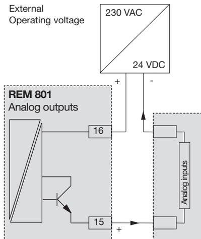
Connection example for the analog output
