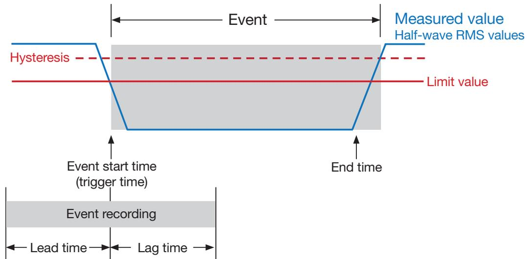
Fig. *Event recording on the REM 801*
