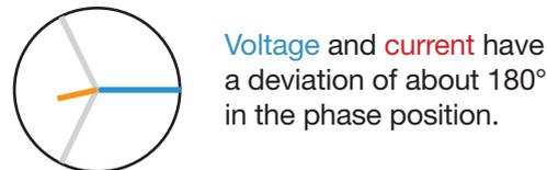
Voltage and current have a deviation of about  $180^\circ$  in the phase position.
