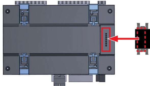
Fig. 2 - Installing the bus connector:
