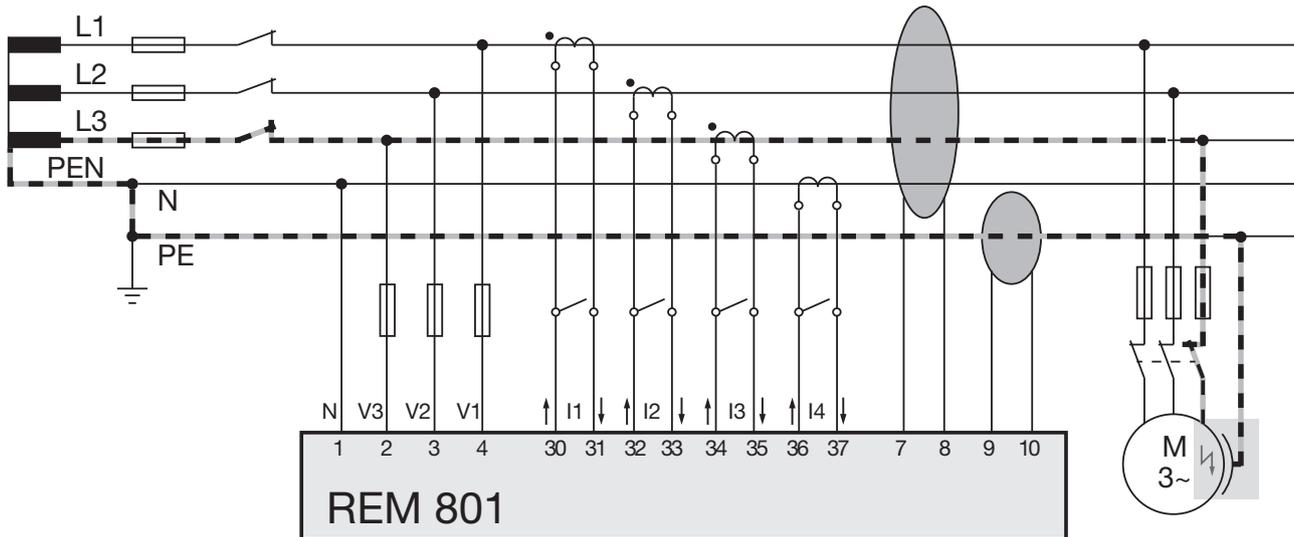
Fig. Connection example REM 801 with residual current monitoring via 2 multifunction channels (7/8, 9/10) as measurement inputs for the residual currents.
