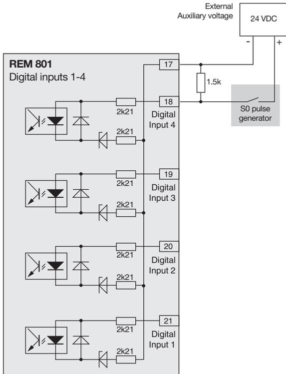
Example for the connection of an S0 pulse generator to digital input 1.
