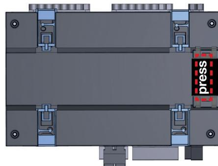
Fig. 3 - Installing the bus connector:
