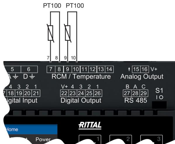
Fig. Connection example "2x temperature measurement" via PT100.
