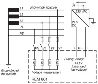
Three-phase 4-conductor network with grounded neutral conductor
