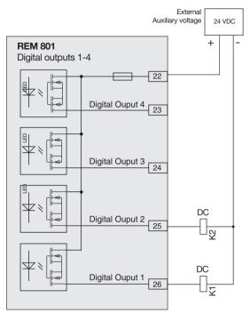
Connection example of two relays to the digital outputs
