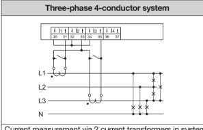
Current measurement via 2 current transformers in systems with the same load.
