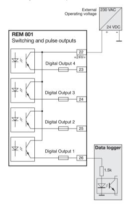
Connection example for wiring as a pulse output.
