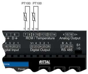
Fig. Connection example "2x temperature measurement" via PT100.
