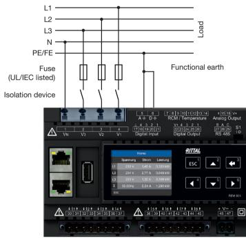
Fig. Connection example for "voltage measurement". PELV
