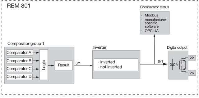
Fig. Application example: Block diagram "Using digital output 1 for limit value monitoring"
