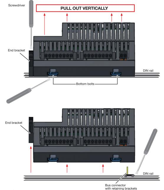
Fig. Dismounting the measurement device
