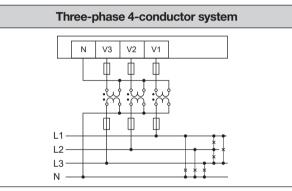
Three-phase 4-conductor system with voltage transformer
