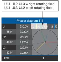
Fig. phasor diagram showing the phase sequence according to the direction of rotating field
