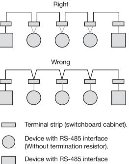
(Termination resistor on the device).
