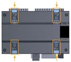
Fig. 4 - Pushing in the bottom bolts: Back of device with bus connector installed and bottom bolts pressed in. (3.) Set up the measurement device with the bus connector on the DIN rail vertically and press until the 4 bottom bolts engage.
