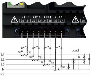
Fig. Connection example for "Current measurement".
