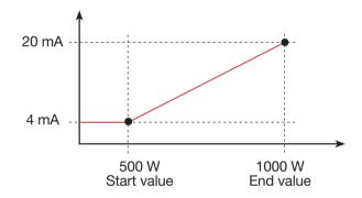
$\cdot$  With an active power of 500 W, the current at the analog output is 4 mA; with an active power of 1000 W --> 20 mA.
