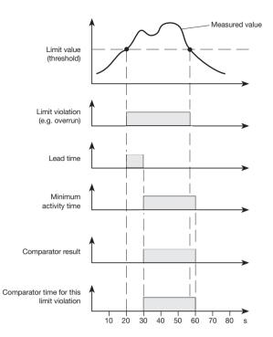
Fig. Comparator without hysteresis Example with 10 s lead time and 30 s minimum activity time
