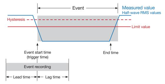
Fig. Event recording on the REM 801
