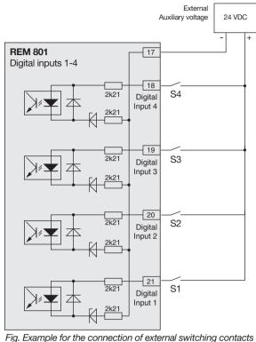
Fig. Example for the connection of external switching contacts S1 - S4 to digital inputs 1, 2, 3 and 4.
