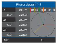
Fig. Window Phasor diagram 1-4
