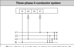
Three-phase 4-conductor system (symmetrical load)
