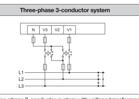
Three-phase 3-conductor system with voltage transformer
