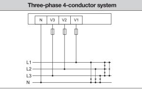
Three-phase 4-conductor system without voltage transformer
