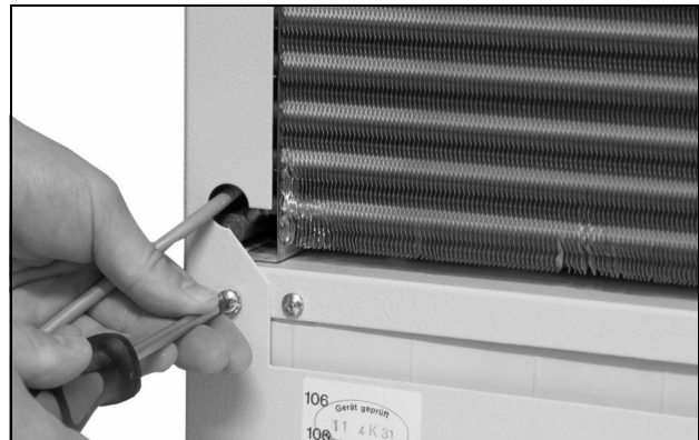
Fig. 28: Remove the assembly screws from the cover (loosen four screws)
