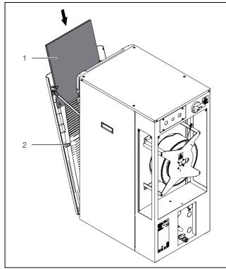
Fig. 39: Slide the filter mat into position 3334400 and 3334450
