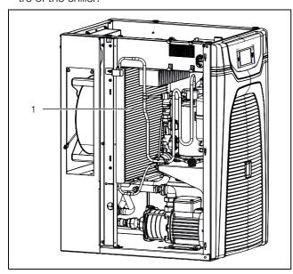
Fig. 51: Cleaning the condenser (shown here: 3334300)
