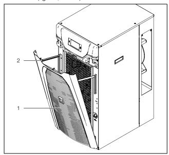
Fig. 38: Flip open the louvred grille 3334400 and 3334450
