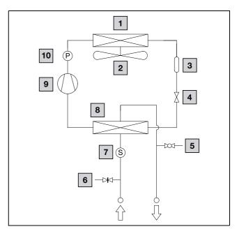
Fig. 18: Schematic diagram of refrigerant circuit with "oil/emulsion"
