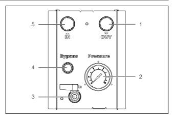
Fig. 20: Device-end connections and display elements
