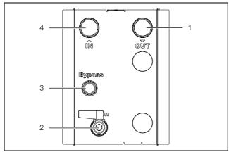
Fig. 8: Device-end connections and display elements
