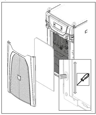
Fig. 35: Insert the textile filter mat 3319100, 3320200 and 3334300
