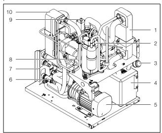
Fig. 22: Components inside the chiller
