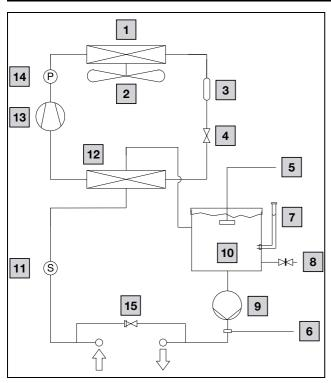
Fig. 9: Schematic diagram of refrigerant circuit
