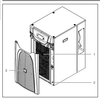
Fig. 34: Pull off the louvred grille 3319100, 3320200 and 3334300
