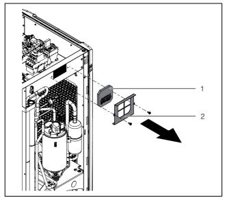
Fig. 40: Pleated filter inverter housing
