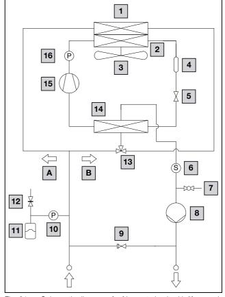
Fig. 21: Schematic diagram of refrigerant circuit with "free cooling" option
