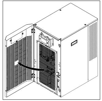
Fig. 15: Swing open the front door
