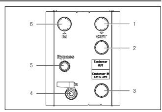
Fig. 23: Device-end connections and display elements
