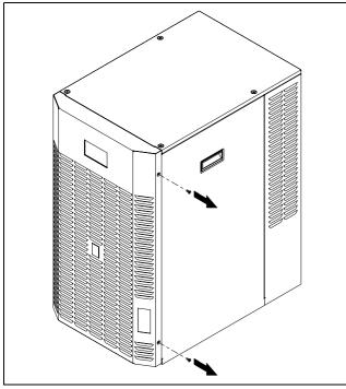
Fig. 14: Remove the locking screws
