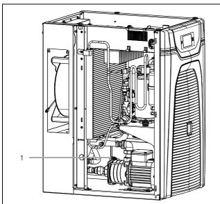
Fig. 42: Bleeding the cooling medium pump
