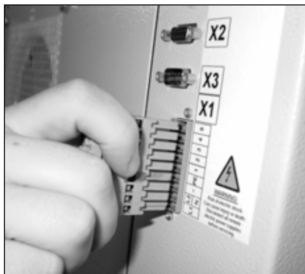
Fig. 27: Disconnect the mains plug
