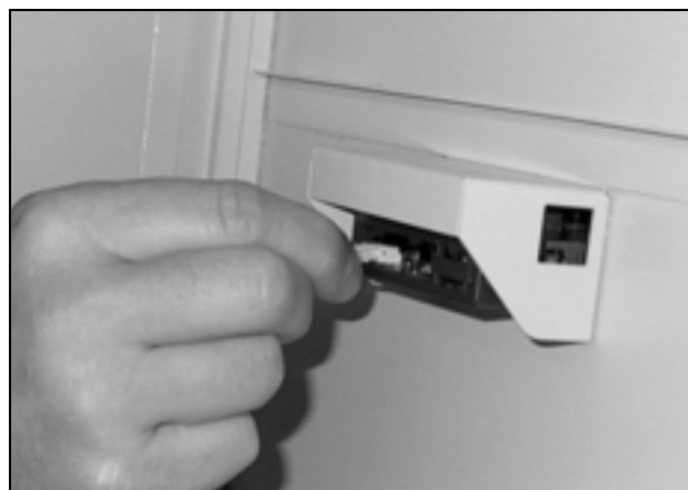
Fig. 28: Disconnect the connector from the display
