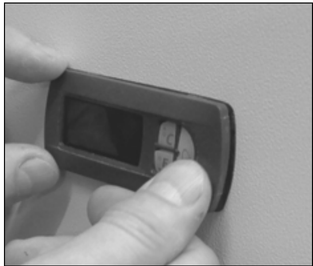
Fig. 12: Attach the trim panel
