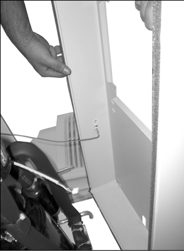
Fig. 72: Disconnect the earthing cable (1)
