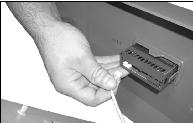
Fig. 60: Disconnect the display cable
