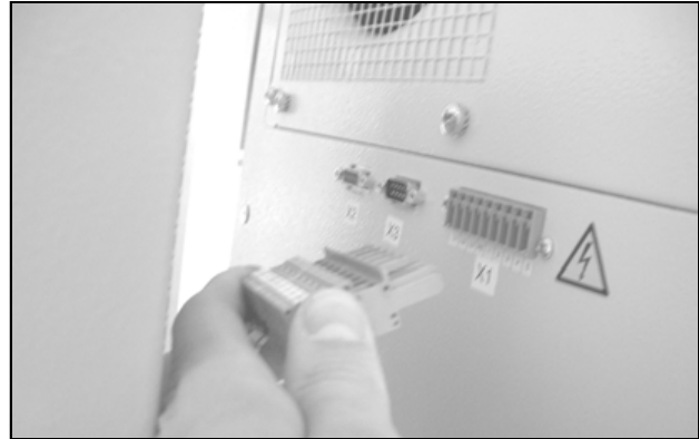
Fig. 53: Disconnect the mains plug
