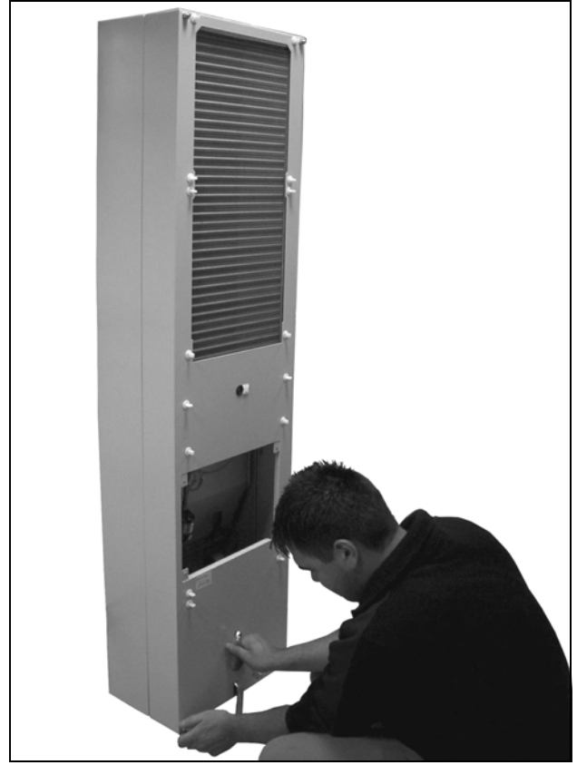
Fig. 70: Undo the four screws for the cover
