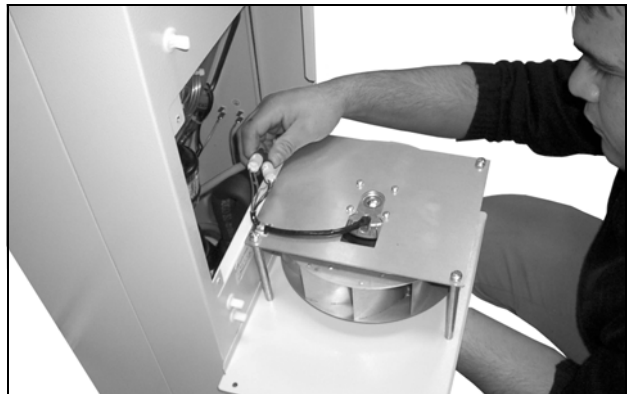
Fig. 65: Disconnect the fan connectors (1)
