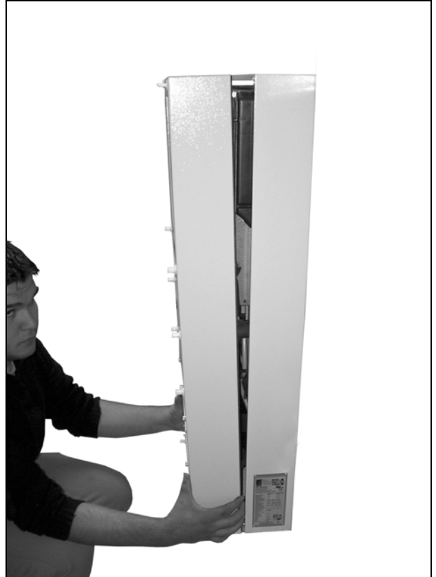
Fig. 48: Remove the cover (2)
