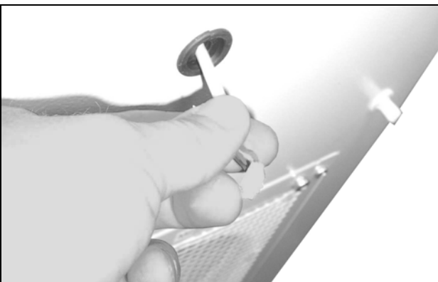
Fig. 61: Slide the display cable back and push it through the cable gland (1)
