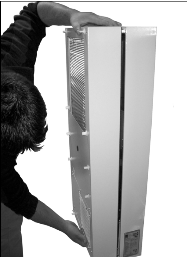
Fig. 47: Remove the cover (1)
