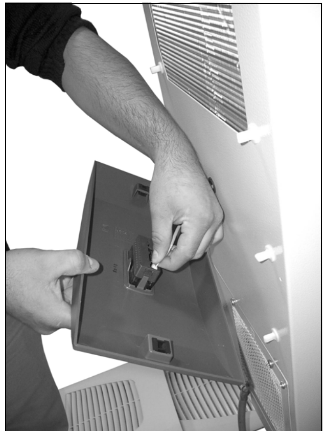
Fig. 38: Disconnect the connector from the display (1)
