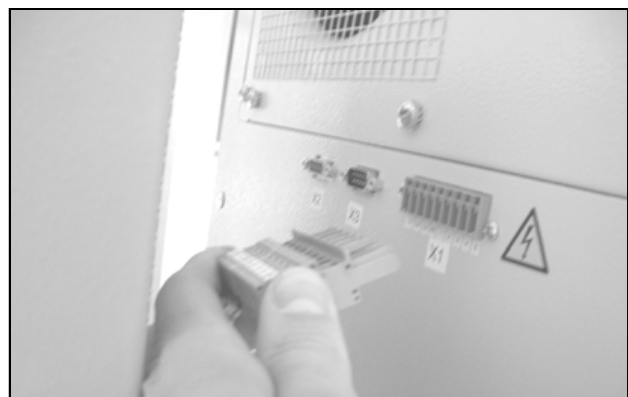
Fig. 34: Disconnect the mains plug
