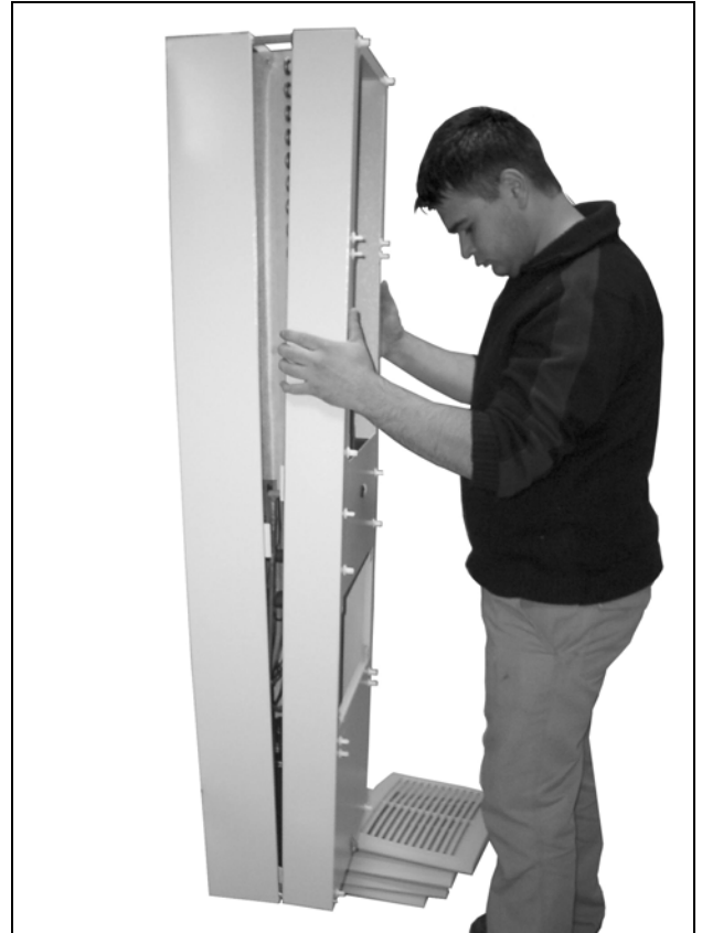
Fig. 71: Removing the cover
