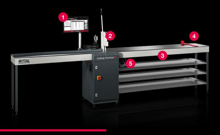
Cut wiring ducts, cable duct covers and support rails to the precise length required with our new Cutting Terminal CT M and Cutting Terminal CT H cutting Terminal CT H variant offers hydraulically supported cutting for support rails.
