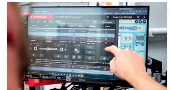
The Eplan Smart Wiring assistance system visualises the mounting layout, devices, connections and wiring routes and acts as a guide for the wiring process.
