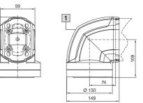
Mounting cut-out, enclosure Ø 130 mm
