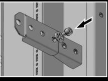
Variable depth adjustment Integrated depth-adjustable attachment for the mounting plate and infill
