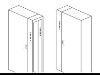
Variable positioning Can be mounted on the left or right
