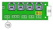
Fig. 11: Connection of external alarm device
