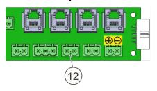
Fig. 12: Manual call point connection
