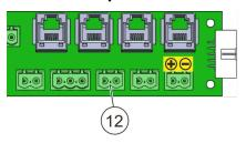
Fig. 39: Connecting terminal "Manual call point"
