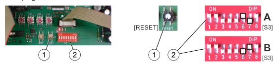
Fig. 35: [Reset] button and DIP switch "S3"
