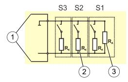
Fig. 40: Manual call points parallel connected
