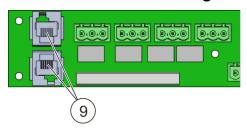
Fig. 15: Connection for networking
