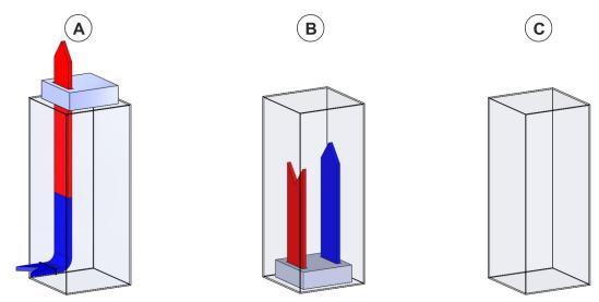
Fig. 16: Cooling air circuit 19" cabinet
