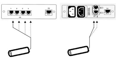
The airflow sensor is installed in the air flow of the fan as required by the sensitivity and the construction type of the fan. If the airflow is below the lower limit, an alarm is triggered. The climate unit in combination with a temperature sensor can use the air flow sensor as control loop for integration in the monitoring setup.. This means no alarm is triggered when the fan stops in normally..
