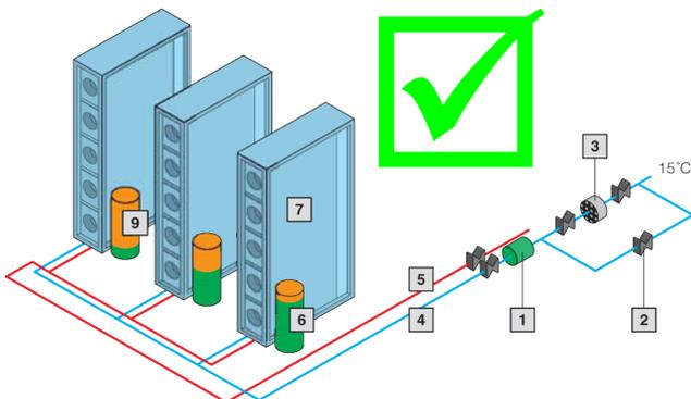
Fig. 23: Cooling distribution with Tichelmann principle
