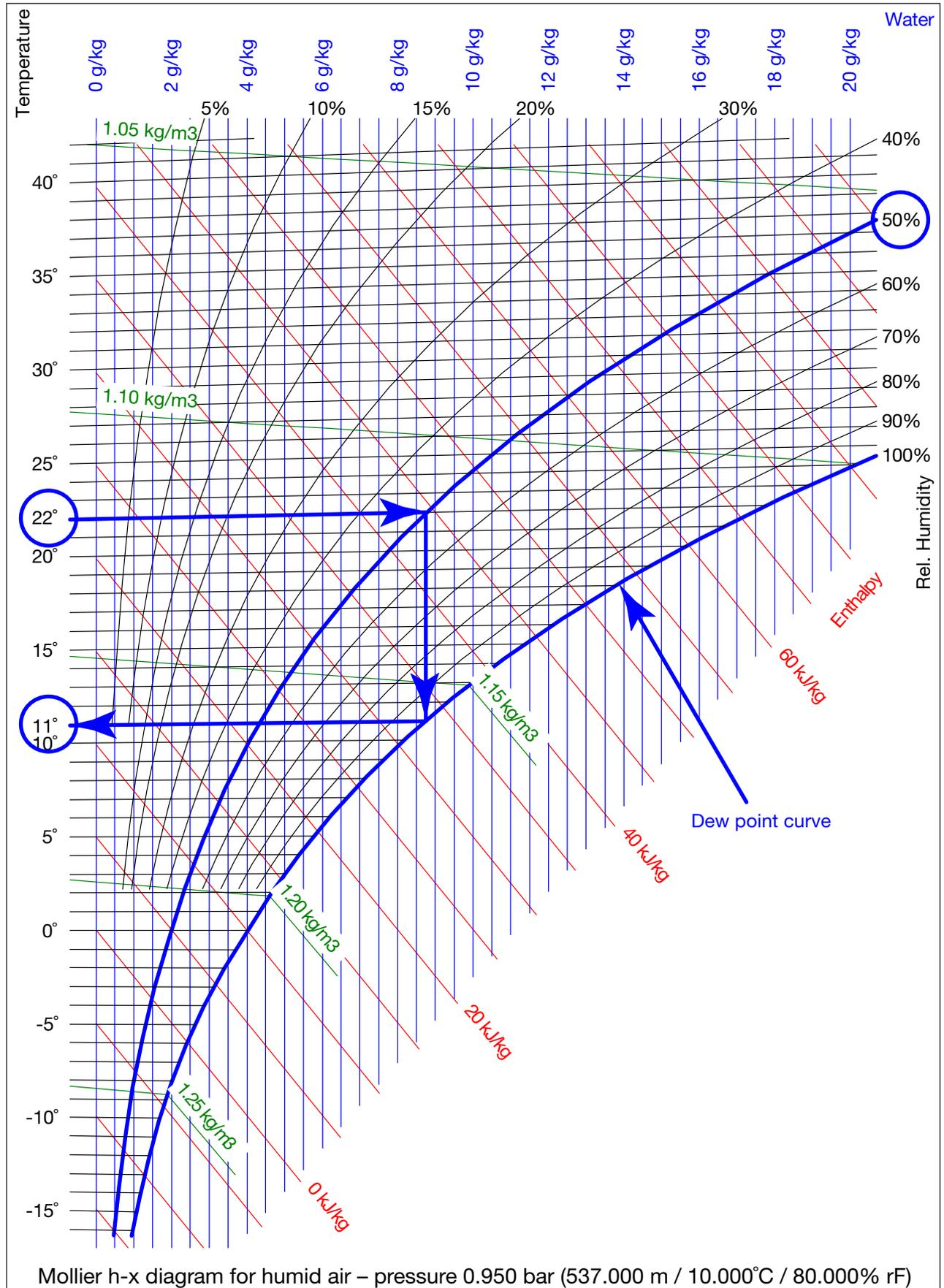
Fig. 2: Mollier h-x diagram for humid air
