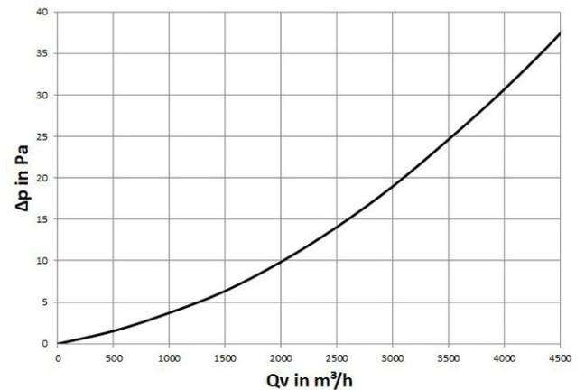
Fig. 29: Airside pressure loss in the "20 kW" version
