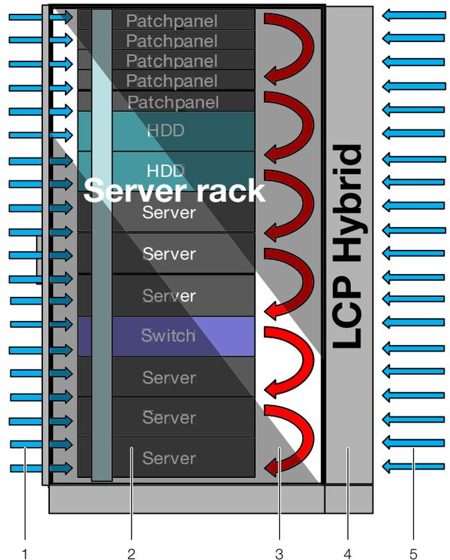
Fig. 10: Incorrect external air stream
