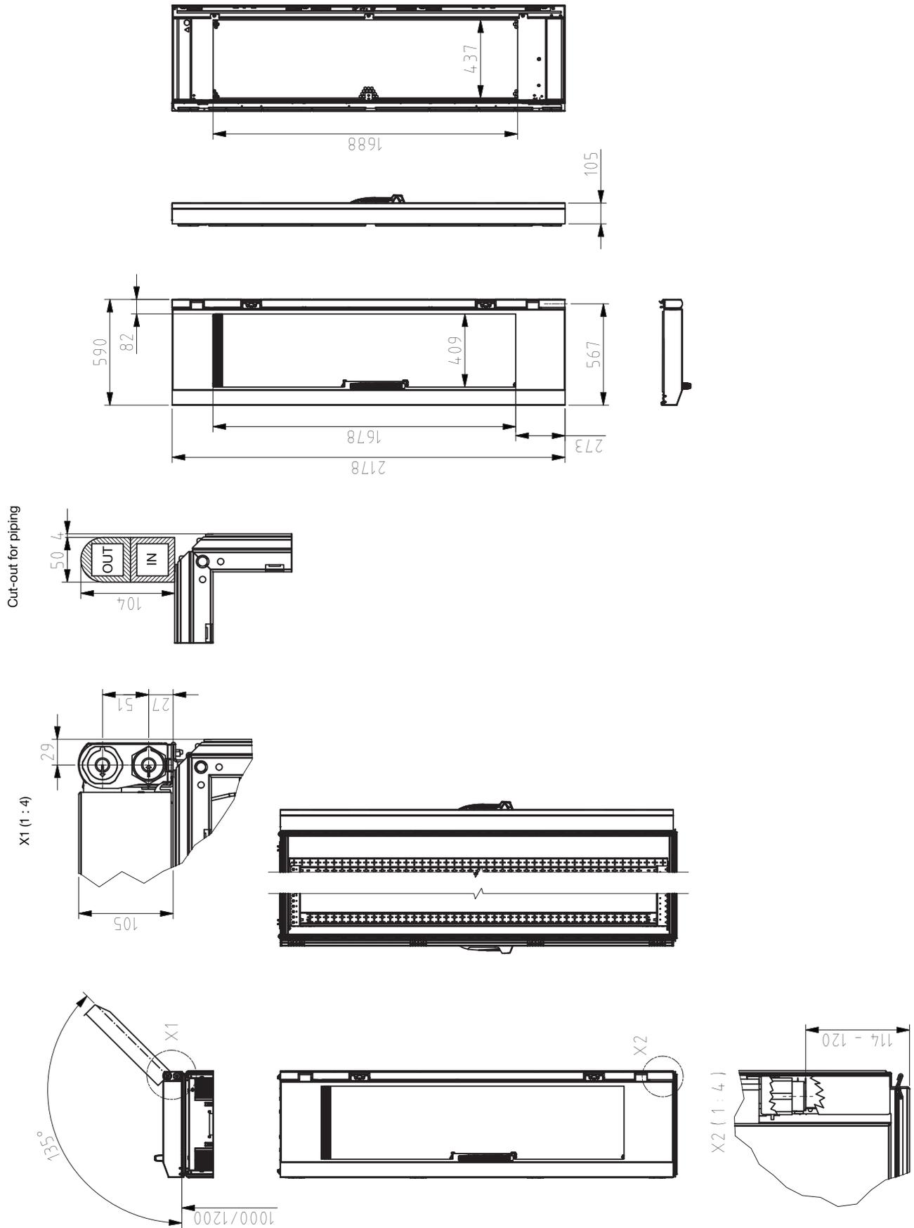
Fig. 34: Overview drawing of LCP Hybrid (600 x 2200)
