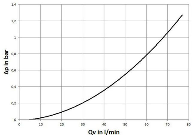
Fig. 30: Upstream pressure loss in the "10 kW" version
