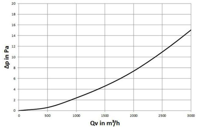
Fig. 28: Airside pressure loss in the "10 kW" version
