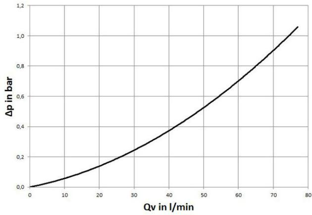
Fig. 31: Upstream pressure loss in the "20 kW" version
