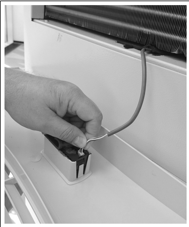
Fig. 24: Disconnect the connector from the display
