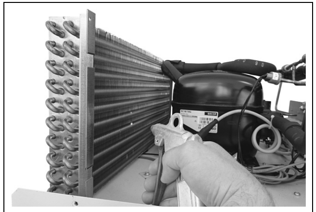
Fig. 30: Clean the heat exchanger coil and compressor chamber using compressed air
