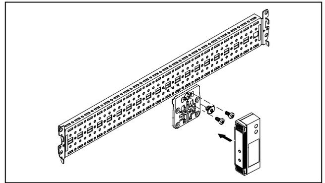
Fig. 7: Fastening the sensor to a system chassis
