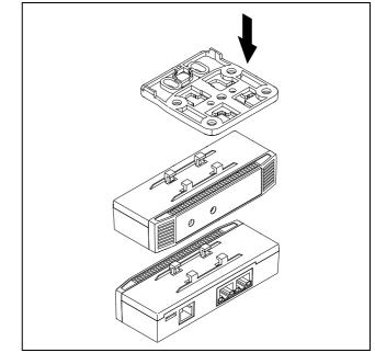
Fig. 3: Attaching the sensor to the bracket
