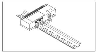
Fig. 9: Sensor with spring clip on the top-hat rail
