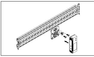
Fig. 7: Fastening the sensor to a system chassis
