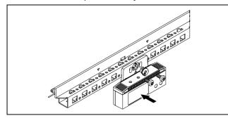
Fig. 6: Optional securing of the bracket
