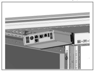
Fig. 2: Faulty installation in the enclosure
