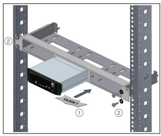
Fig. 7: Fastening the mounting unit in a rack-mounting point
