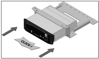
Fig. 4: Push the I/O unit into the mounting unit
