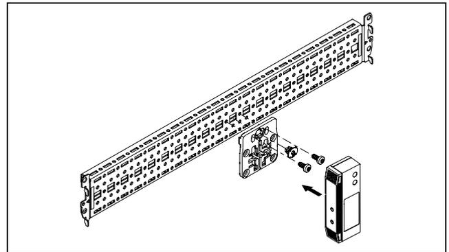
Fig. 7: Fastening the sensor to a system chassis
