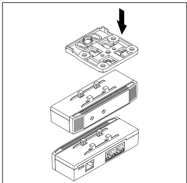
Fig. 3: Attaching the sensor to the bracket
